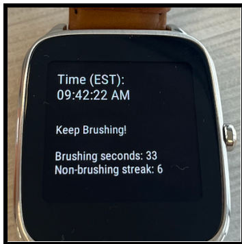
Fig. 1. Photo of running smartwatch sensing application on Asus ZenWatch 2.
